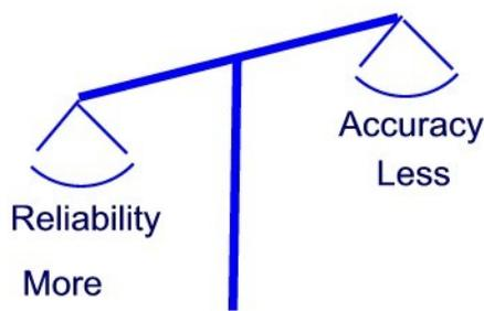
The two detector log counts both epithermal and thermal neutrons. It does this so that a meaningful populations of neutrons can always be counted. This makes the log reliable in a sense, but creates an inaccuracy problem, because the thermal neutrons population has been reduced by capture/absorption making the hydrogen index less accurate.
