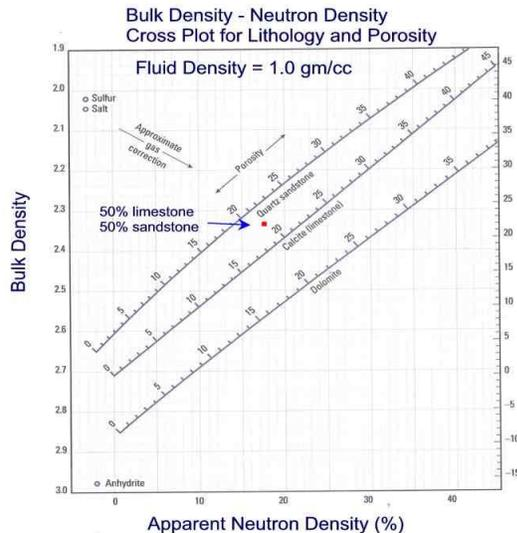
The M/N lithology plot is used to identify a complex mixture of sandstone, dolomite and limestone using all three porosity logs. The rationale for the M/N plot is that the porosity should be the same in all three porosity logs for the same composition of lithology.
