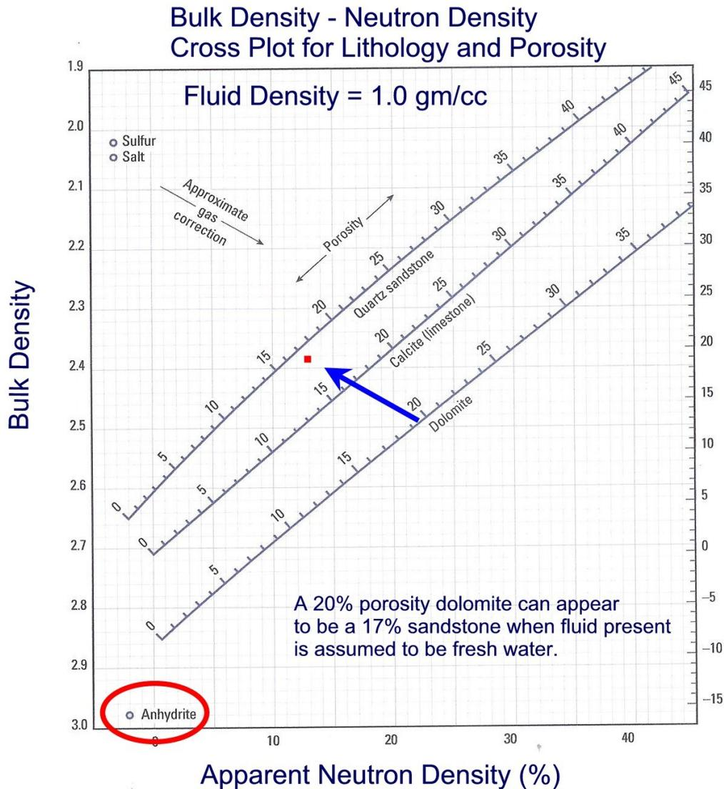
Also note that evaporites are clearly identified both by the bulk density and the apparent neutron density of approximately zero.
