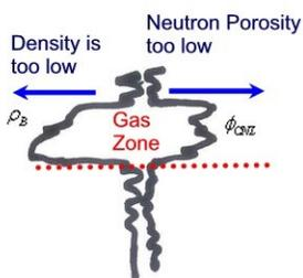
In limestone and dolomites, the lithology of a gas zone may show up as a sandstone (a move up and to the left). The correction for gas is then down and to the right. The gas contact can sometimes be easily identifiable in carbonates from the raw logs, as they are frequently plotted on a limestone scale ( $\phi_{CNL} = 0$ ,  $\rho_B = 0$ ). The gas will cause the density log to be abnormally low, at the same time, the neutron porosity will read too low.
