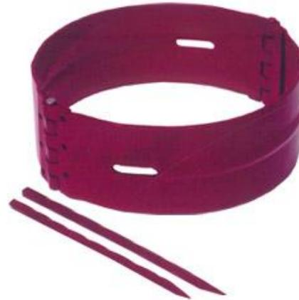
The number of centralizers to be run is based on an American Petroleum Industry standard of at least a 70% standoff ratio. A perfectly centered well would have 100% standoff, and a well string touching the side of the formation would have zero standoff .
